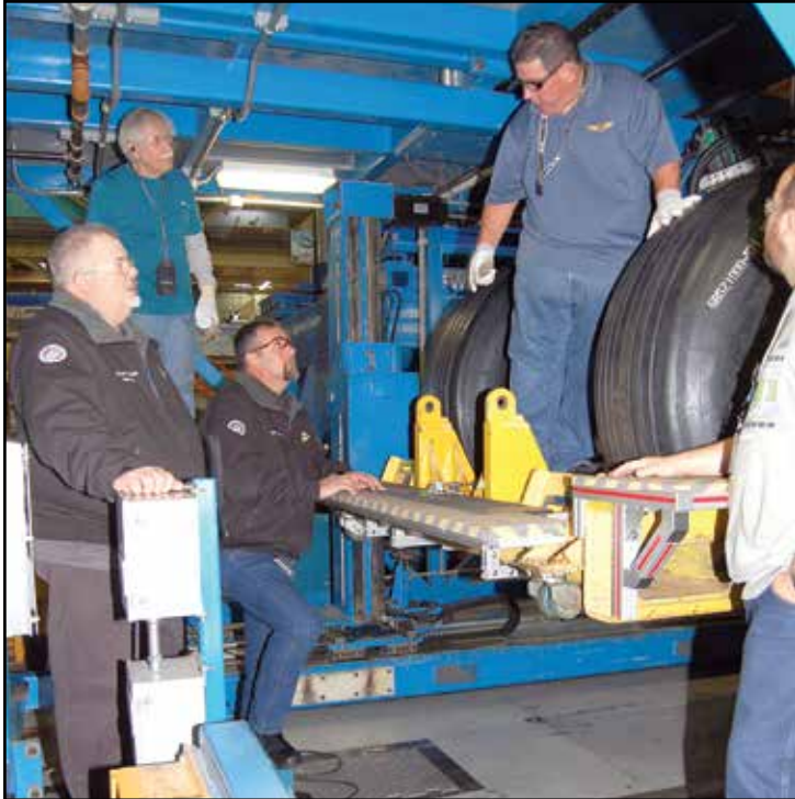
L to R: Business Rep Howard Carlson, Jim Riveira, Joint Programs Coordinator John Kussy, Brian Butler and Andrew Dennis examine the new 18-inch platform to remove the 787 landing gear tool rather than balancing on a 4-inch beam.
